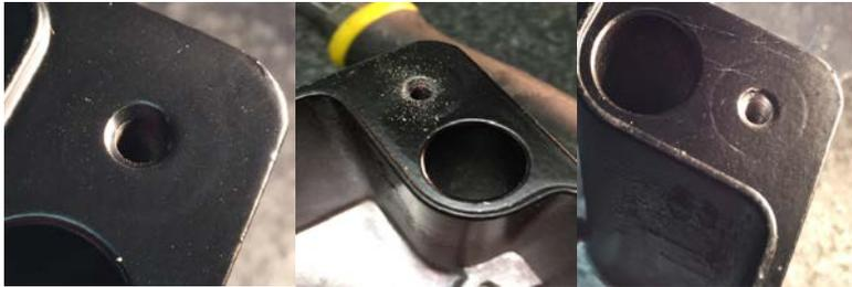
3- When dealing with a painted box, there may be some powder in the threads; this requires over torquing the screws (can get to 28 in\*lb). It is best to move in and out a couple of times with each screw to release friction.
