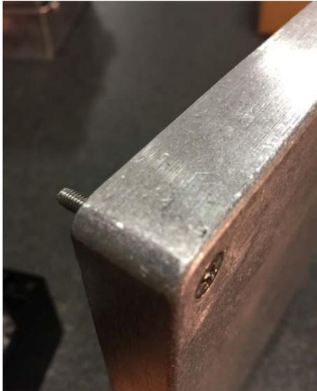
1-Captive screws must be screwed in the **cover first** (screw should drop once past the threaded area)
