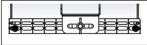
4. Mount the corner bracket (15101-CB) onto a corner of two walls using the 2 supplied #8 x 2" drywall screws according to the mounting orientation you have chosen (the bracket should overlap with the enclosure back) . with heavy enclosures it is recommended to use the additional holes in the bracket.
