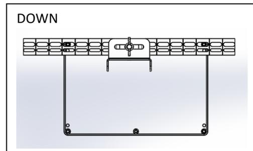
3. Assemble 2 enclosure mounting screws (not supplied) to secure the strip to the enclosure, and use your hand to break off any parts of the strip that are sticking out of the sides of the enclosure.
