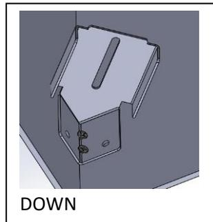
5. drop the 1/4" carriage bolt in the square hole in the tray (it is recommended to use a piece of tape over the bolt's head to temporarily keep it from moving up) and assemble the tray to the corner bracket using one one 1/4" wing nut, paying attention to place the nut on the corner bracket side.
